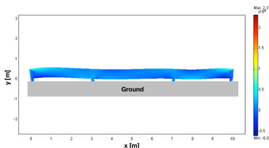
Fig. 4. Simplified FE model of the headstock structure of the reference machine under thermal and structural loads.
