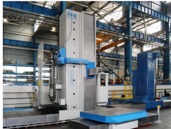
Fig. 1. PAMA SpeedRam 2000 CNC Milling/boring machine (travels: headstock 5 m, column 4 m, ram 1.2 m, spindle 1 m).
