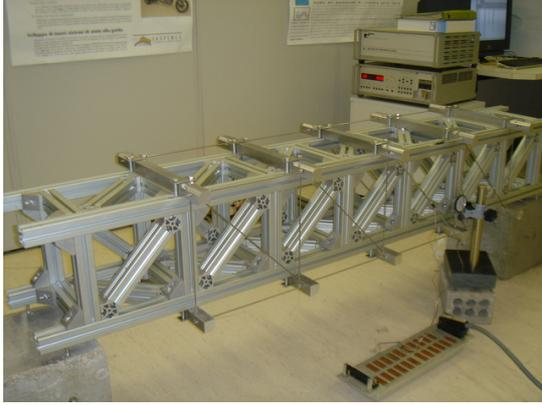
Fig. 8. Test bench with a four-meshes SDD prototype. A digital dial indicator used during the test is visible near the lower left corner of the picture.
