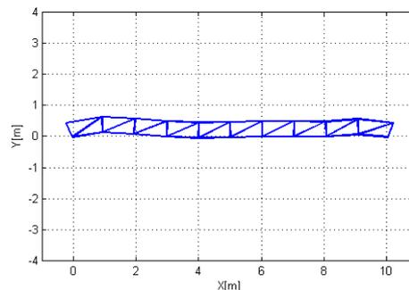
Fig. 5. Deformed shape of the reticular sensor (deformations magnification factor: 1000).
