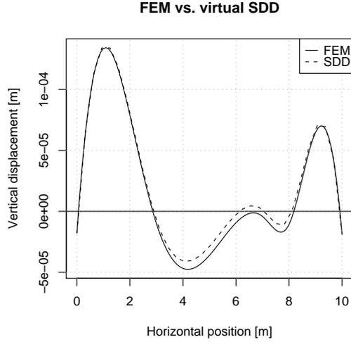
Fig. 6. Vertical displacement of the reference structure as a function of the horizontal position, as calculated by FE model and by the virtual SDD (strain resolution:  $1 \times 10^{-6}$ ).
