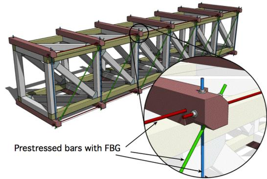
Fig. 7. Concept model for a test bench: a reticular beam with a superimposed grid of FBG sensors in horizontal, vertical, and  $45^\circ$  direction.
