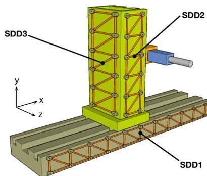
Fig. 2. Simplified model of a large milling machine (typical travels as for Fig. 1). Three reticular SDD sensors are shown on horizontal and on vertical elements.
