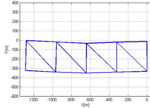
Fig. 9. Deformed shape for the test bench under vertical load applied at the middle span, as computed by the SDD (exaggerated).
