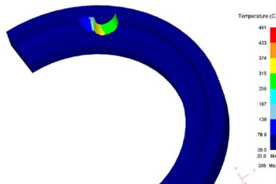
Fig. 2 – Milling simulation of titanium alloy, for cutting speed of 157 m/min, feedrate of 0.1 mm/tooth and depth of cut of 1mm
