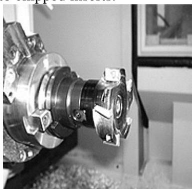
Fig. 3 – Multi tooth milling tool
