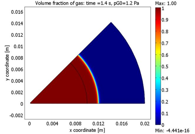
**Figure 2.** Growth of a gas bubble in a liquid corresponding to the simulated case b) of section 3.
