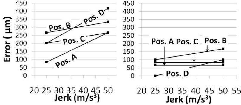
Fig. 9. Maximum circular error during the STAR a) 10 m/min, b) 5 m/min (SPARK)
