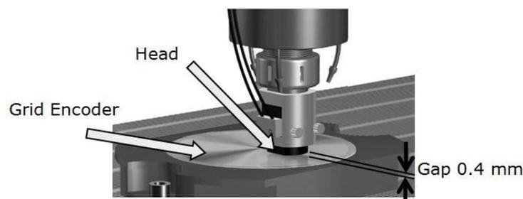
Fig. 1. Components of the grid encoder HEIDENHAIN KGM182
