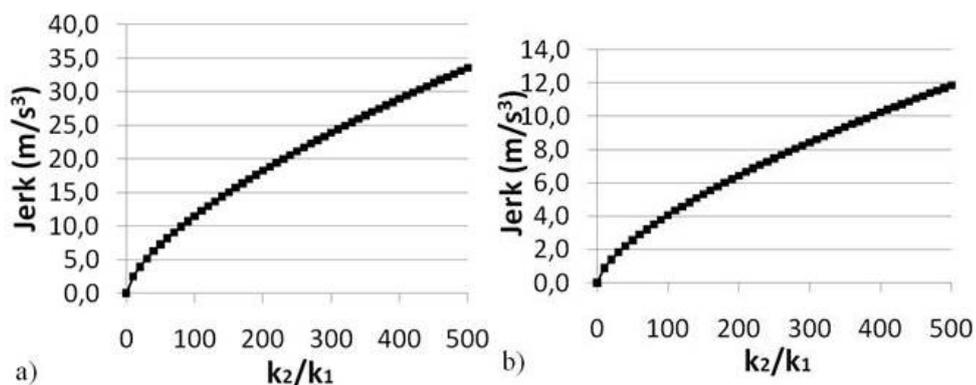
Fig. 12. Plot of the optimal Jerk vs. the ratio  $k_2/k_1$ , with  $D = 1.05$  a) with  $D = 5$  b) (SPARK)
